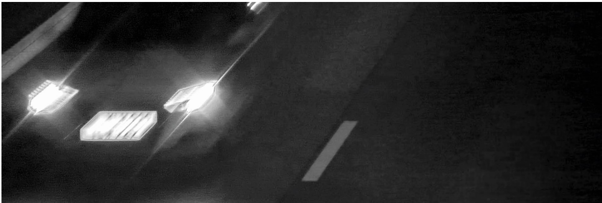
Figure 13. A car moving at high speed is imaged with a shutter time of 1/30 s.
