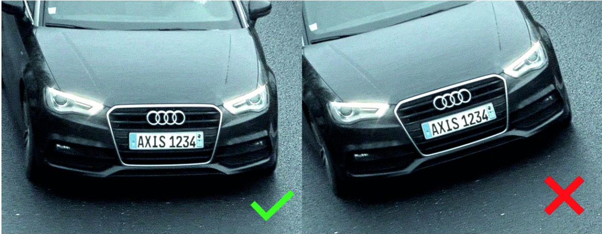
Figure 10. The camera should be aligned so that the license plate is parallel to the edge of the image.
