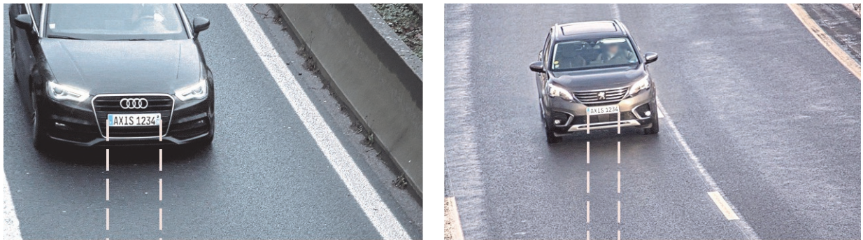
Figure 6. The number of pixels across the width of the license plate depends on the camera resolution and the scene width. In this example a camera with a resolution of 1080x1920 pixels is (left:) zoomed in on one lane (4 m wide) and (right:) zoomed out to cover almost two lanes (6.5 m wide). The license plate covers 250 pixels and 154 pixels, respectively.
