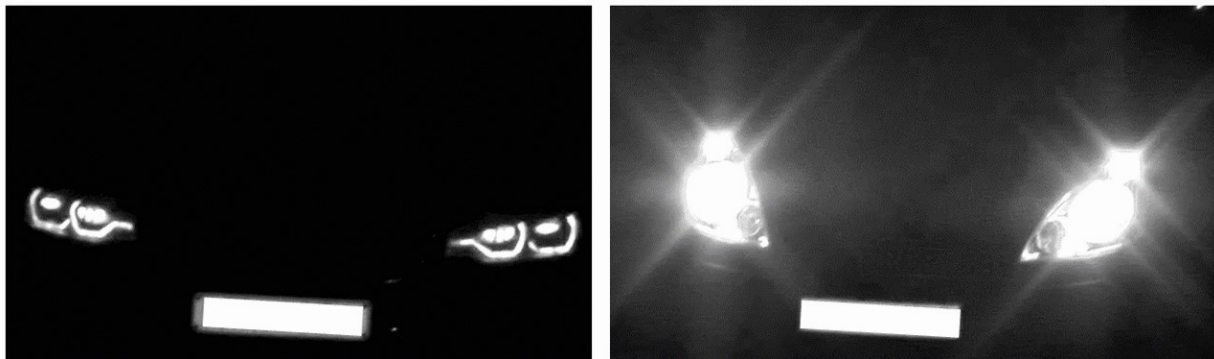
Figure 16. Left: the light from LED headlights is blocked by the IR-pass filter, which efficiently reduces lens glare and stray light. Right: the light from halogen headlights goes through the IR-pass filter and gives rise to lens glare. The two images were taken almost simultaneously, with identical settings and alignment, using a camera equipped with an IR-pass filter.
