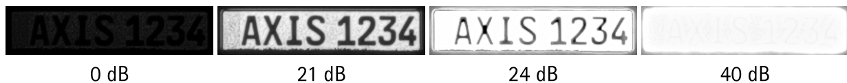
Figure 14. The max gain setting will determine how the license plate is exposed at night.
