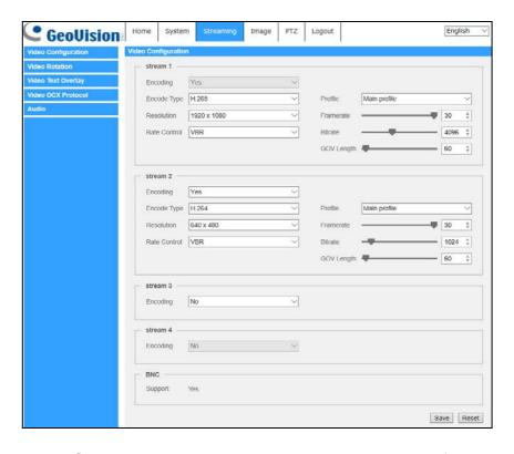
In the Streaming submenu, the administrator can configure specific video resolution, video compression mode, video protocol, audio transmission mode, etc. Further details of these settings will be specified in the following sections.
