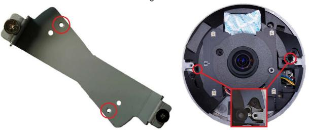
3. Fasten the two supplied M3x18 mechanical screws at the two aligned holes to fix the camera to the In-Ceiling Plate.
