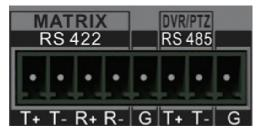
Figure 4-15 RS-485 Serial Port
