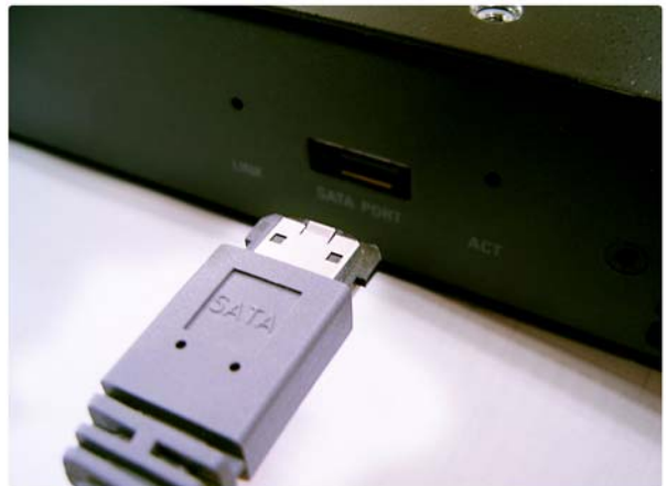
Connecting the SATA cable which letters must be top side
