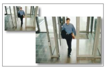
The increased resolution can also be used to provide a significantly larger overview. The inner rectangle below shows the area covered by an analog high-resolution camera. With the same number of pixels per area, the full 1280x1024 resolution provided by AXIS 211M - the outer rectangle below - covers a three times larger scene.
