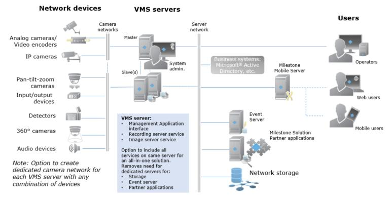
A single **Management Application interface** provides a single point of access to Recording Servers. System configuration wizards help add cameras, configure video and recording, adjust motion detection and configure multiple users.
