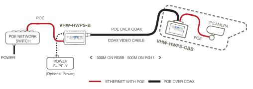
HIGHWIRE Powerstar Backbox delivers Ethernet and POE over legacy coax, for maximum reliability with minimal wiring.
