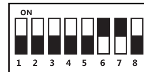
DIP Switch of Wiegand 26 Protocol
