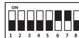
DIP Switch of Wiegand 26 Protocol
