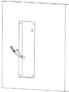
Figure 2-38 Cave the Installation Hole
