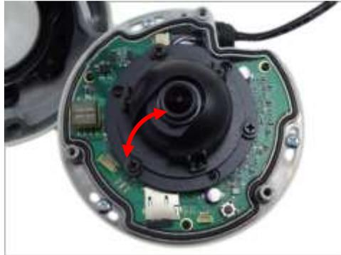
**NOTE:** Because the lens is secured tightly to the module, users need to push hard to tilt the lens.
