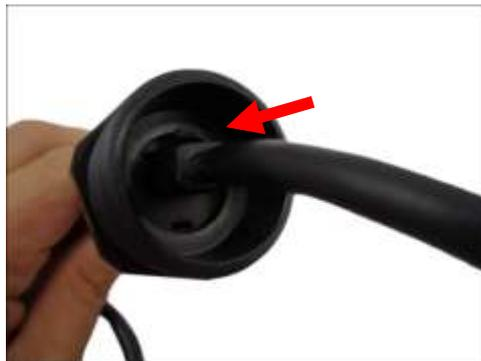
7. Insert the sealing rubber and claw into the cable gland body.
