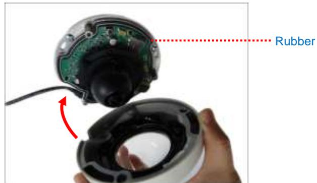
**NOTE:** Make sure the rubber on the camera is positioned properly on its track as the dome cover is closed on the camera to ensure protection against water ingress.
