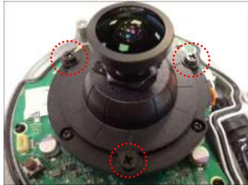
3. Turn the lens module to adjust the viewing orientation. The arrow on the lens indicates the top side orientation.
