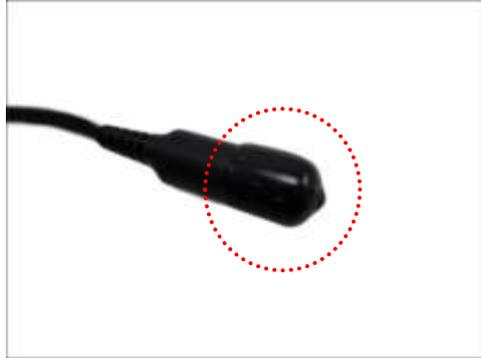
**WARNING:** Do not remove this rubber protection if the audio-in jack will not be used to avoid water or dust from entering the jack.
