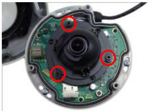
5. Push the lens up or down to adjust to preferred tilt.
