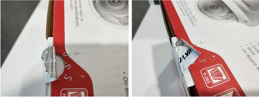
Figure 2 Tamper seal sample after a tampering attempt
